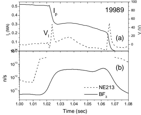
Figure 1: A plasma disruption showing the formation of a 0.3 MA runaway current: (a) Plasma current (full line) and loop voltage (dashed line) traces; (b) Neutron measurements:  $BF_3$  (full line) and NE213 (dashed line) signals.
