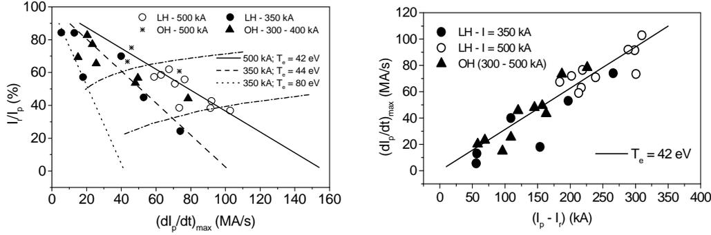
Figure 2: **Left:** For the analyzed FTU runaway current plateau disruptions: Fraction of runaway current vs maximum current derivative during the disruption current quench; **Right:** Maximum current derivative during the disruption current quench vs  $I_p - I_r$  (data for OH disruptions from previous campaigns have also been included for comparison).
