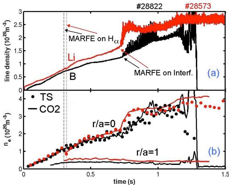
**Figure 3.** a) Central chord of line integrated density Boronized and Lithized discharges. Oscillations at 0.7 s are due to an extended MARFE present at the edge. Vertical lines mark the time when MARFE appears on  $H_\alpha$ . b) central and peripheral density for the same discharges. TS central density is also reported for comparison (full circles).
