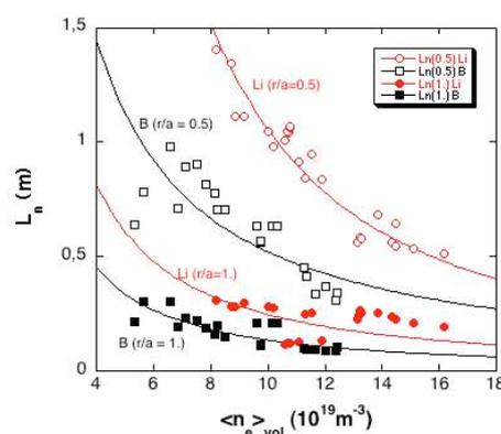
**Figure 5.** density profile characteristic length for discharges with marfe, at half radius (open marks) and edge (full marks).
