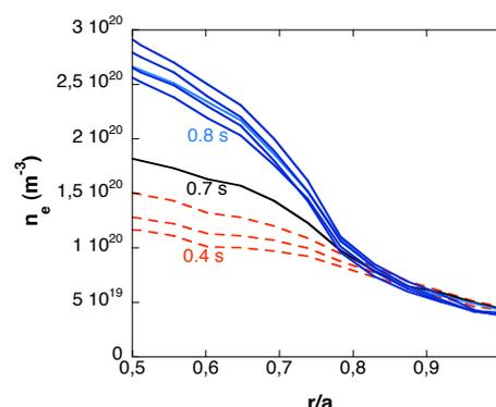
**Figure 4.** Density profile evolution in a discharge with marfe. Marfe appear at 0.7 s.
