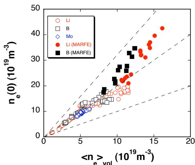
**Figure 2.** Peak density versus volume average density. Black squares for boronized wall, red circles for lithitized and blue diamonds for metallic. Full marks are for discharges with MARFE. Straight lines are constant peaking factors 1, 2, and 3.
