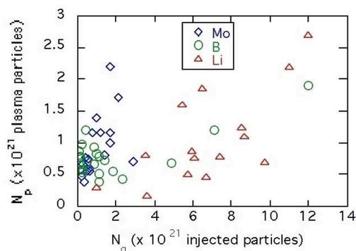
Figure 1. The total plasma particles  $N_p$  versus the total amount of injected particles  $N_g$
