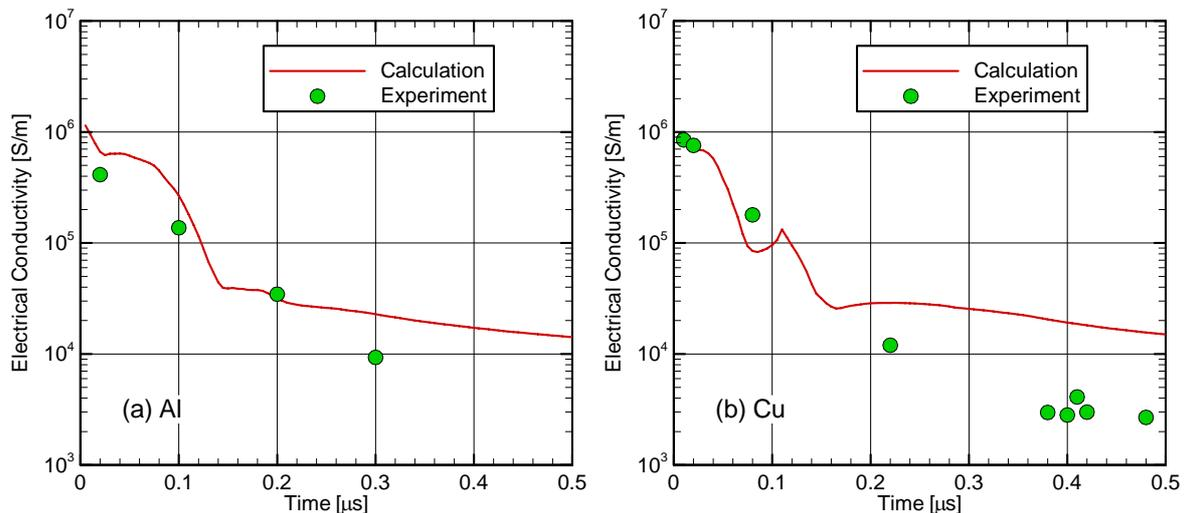
FIG. 3. Electrical conductivities of (a) aluminum and (b) copper plasmas during the Joule heating stages.
