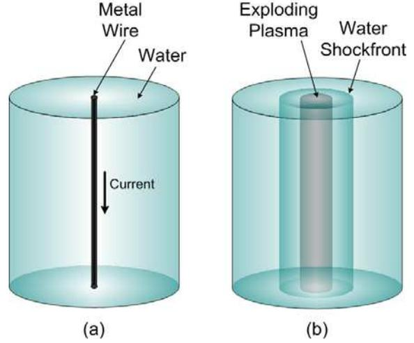
FIG. 1. Schematic diagram of metal wire explosion in water (a) before and (b) after discharging.
