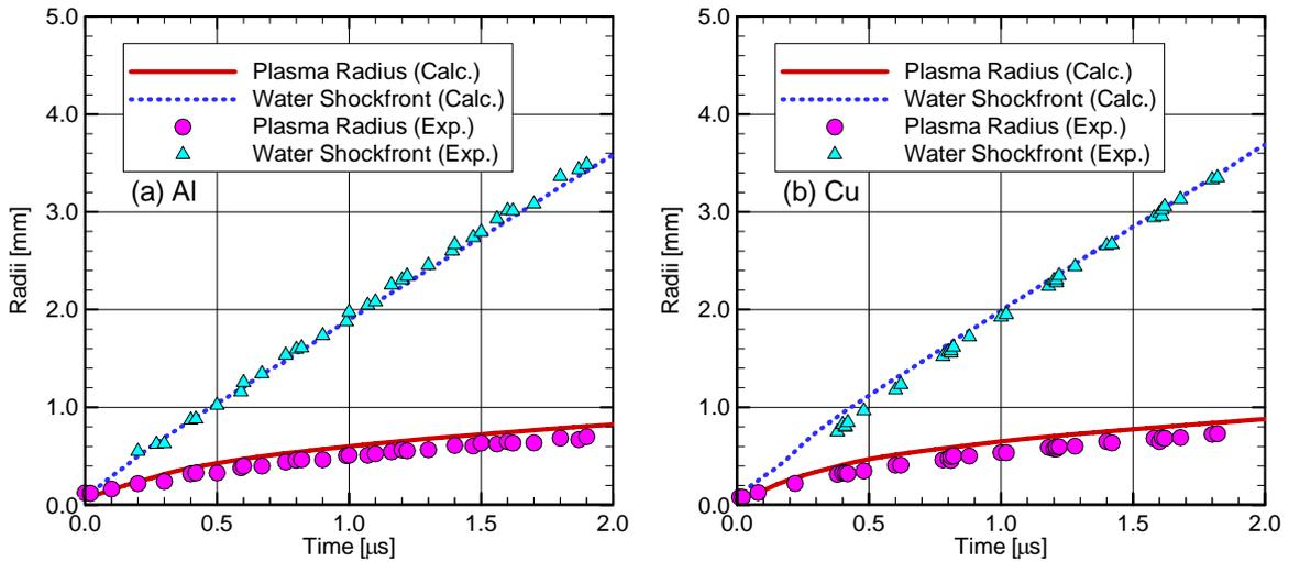
FIG. 2. Calculated trajectories of plasma column radii and water shockfronts of (a) aluminium and (b) copper wires.
