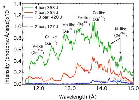
**Figure 2:** Xe X-ray spectra as a function of gas pressure and laser energy.
