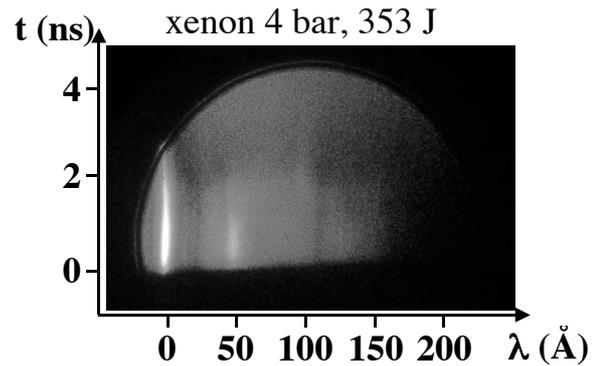
**Figure 3:** XUV streaked image recorded at 4 bar gas pressure. The wavelength origin is settled on the zero order.
