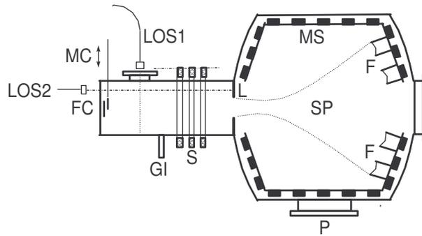
**Figure 1 : MISTRAL-B experimental device.** SP: source plasma ; F: filaments ; MS: ferrite magnets ; P: pumping system ; L: limiter ; S: solenoid ; GI: gas injection ; FC : fixed collector ; MC : moving collector ( $\Delta V$ ); LOS1 : line of sight 1 (radial observation of central plasma) ; LOS2 : line of sight 2 (axial off-axis observation of the ejected plasma).
