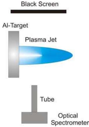
Figure 1: Schematic setup of the optical spectrometer
