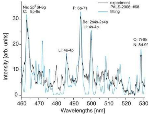
Figure 2: Experimental spectrum (black curve) from aluminium. Some line transitions are indicated. The blue curve shows a fitting (see text).
