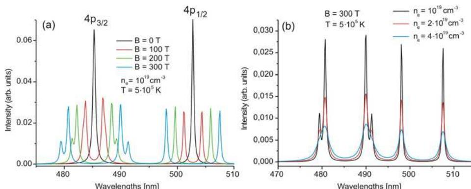
**Figure 4:** Simulations of combined Zeeman/Stark effect Li-like 4s-4p transitions of Al
