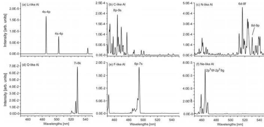
Figure 3: Theoretical spectra ( $F_{ii}=1$ ) of aluminum originating from various
