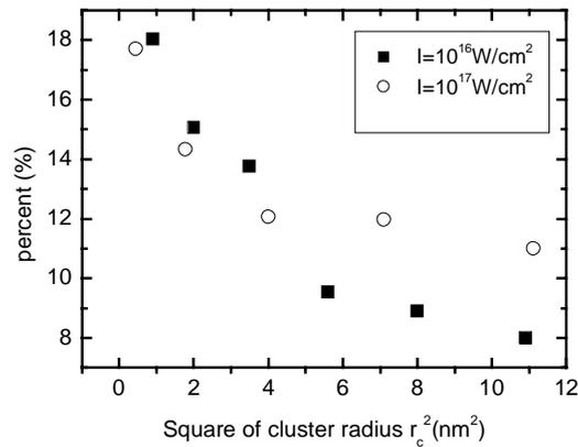
Fig.4, Dependence of the percent of  $H^+$  only to the total distribution on the square of cluster radius  $r_c^2$  (nm<sup>2</sup>) at  $1 \times 10^{16}$  W/cm<sup>2</sup> and  $1 \times 10^{17}$  W/cm<sup>2</sup>.
