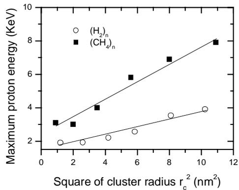
Fig.2. Dependence of the maximum proton energy  $E_{\text{max}}$  of the exploding on the square of the cluster size  $r_c^2$ .
