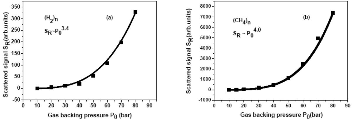
Fig.1 Rayleigh scattered light signal  $S_R$  as a function of the gas backing pressure  $P_0$  (a) for the hydrogen clusters, and (b) for the methane clusters. A nozzle with a  $300\mu\text{m}$  orifice used.
