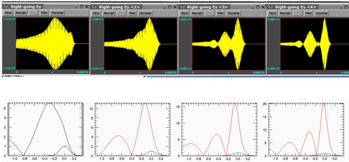
Fig.2 Evolution of a pulse. The top row shows the time evolution from a particle-in-cell code, while the bottom row shows the corresponding results from the analytic approximation. The initial pulse is also shown in the bottom set of graphs.
