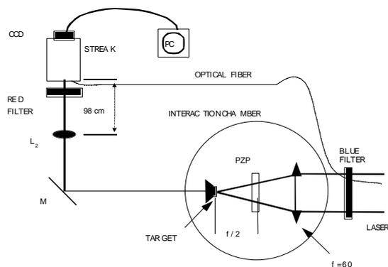
Figure 1: Experimental set-up at PALS.
