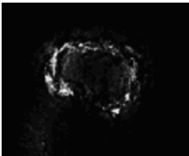
Fig. 1a. Top view of the Crater on aluminium target.
