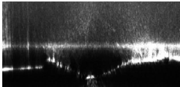
b. Reconstructed crater profile corresponding to the crater in fig.1a. Depth is 85  $\mu\text{m}$ .
