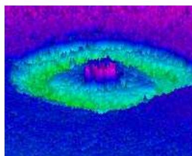
Fig.4.  $\sim 350 \mu\text{m}$  diameter crater on Al-target. M=800.
