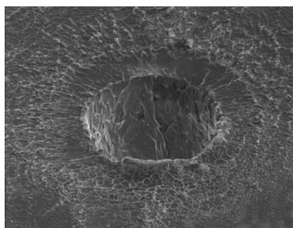
Fig.3.  $\sim 90 \mu\text{m}$  diameter crater on Al-target.
