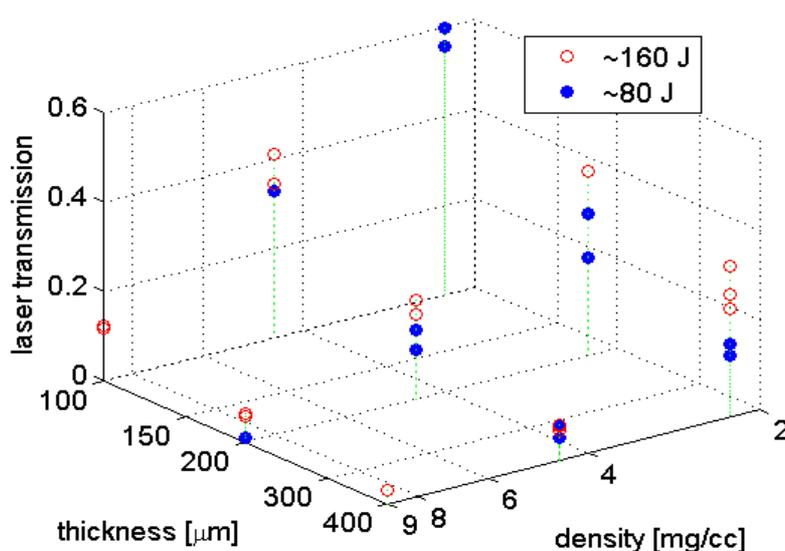
**Figure 2:** Laser transmission through foams of various densities and thicknesses. Laser pulse of energy in the range of 153 – 183 J (open circles) and of 74 – 88 J (filled circles), of wavelength 439 nm and of duration 320 ps was incident normally on the foam target, best focus was 500  $\mu\text{m}$  ahead of target and laser spot diameter on the target was 300  $\mu\text{m}$ .
