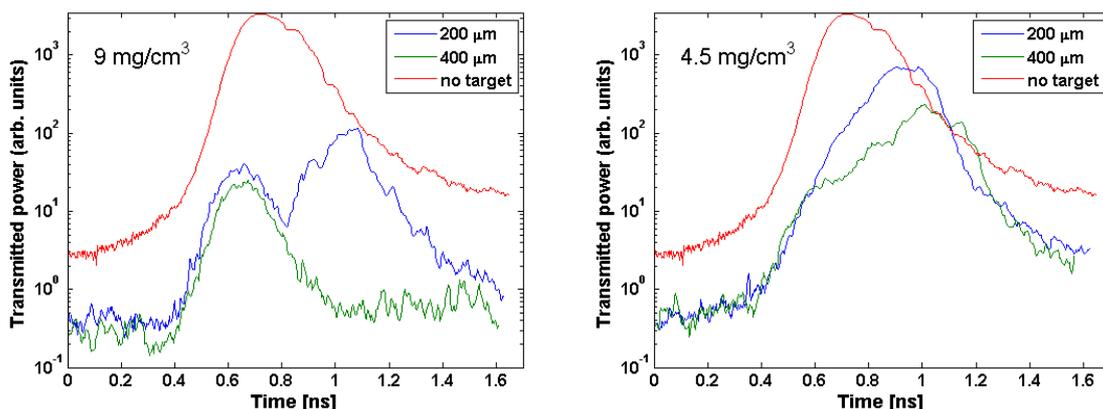
**Figure 1:** Laser transmission through foam layer compared to vacuum transmission. Laser pulse of energy in range 150 – 170 J, wavelength 439 nm and duration 320 ps is incident normally on TAC foam layer of thickness 200 or 400  $\mu\text{m}$ . Foam density is 9 and 4.5  $\text{mg}/\text{cm}^3$  in the left and right graph, respectively.
