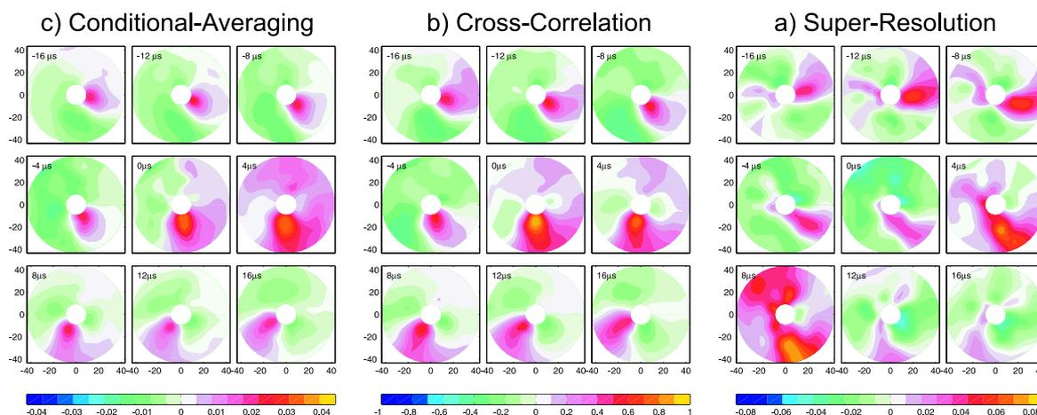
Figure 3: Snapshots on weak turbulence evolution in the KIWI experiment using: a) CA having the reference signal situated to the maximum amplitude fluctuations at about  $\tau=4\mu\text{s}$  b) CA having similar reference signal c) Super-Resolution. The color bars encode the absolute amplitude value with exception of CC. There, it represents the value of the cross-correlation function.
