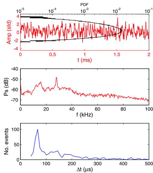
Figure 2: a) The normalized reference signal and probability density function (PDF) b) power density spectrum (Ps) c) the events statistics of the reference signal in CA processing
