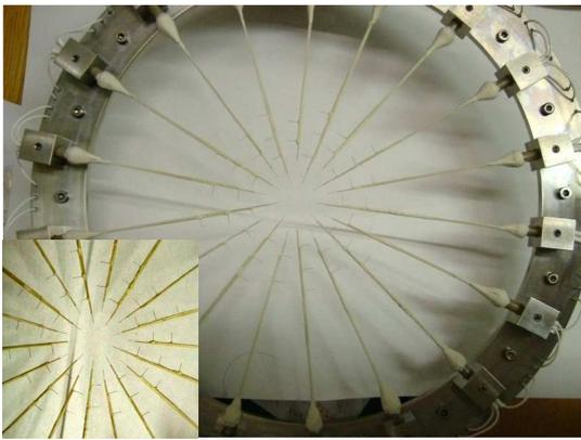
Figure 1: Picture of the 2D probe array. The 63 Langmuir probes are adjusted for a uniform spatial distribution.
