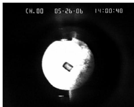
Figure 3. In-flight picture of a 3 mm D<sub>2</sub> pellet, travelling at about 1.2 km/s.
