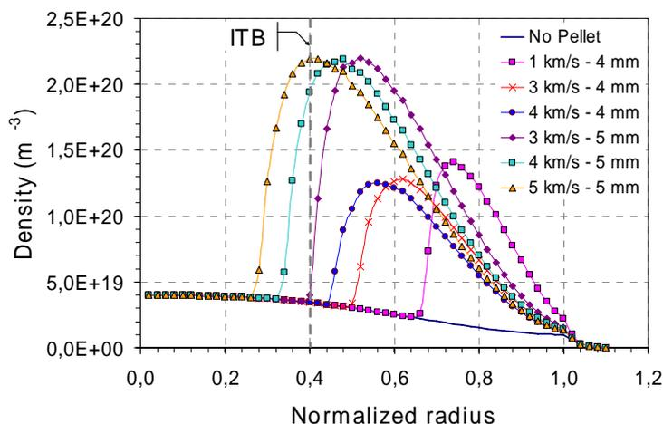
Figure 4. Estimated penetration depth in JET of D<sub>2</sub> pellets (4 to 5 mm size range) injected in the midplane from the LFS
