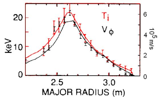
Fig. 2. Impurity ion temperature and drift velocity in TFTR. (N.B.: here  $T_i$  is our  $T_x$ .)
