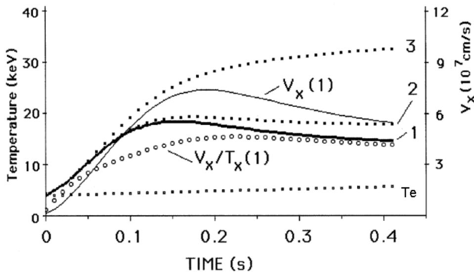
Fig. 3. Calculated toroidal drift and temperature of  $C^{6+}$  ions in a TFTR NBI plasma.
