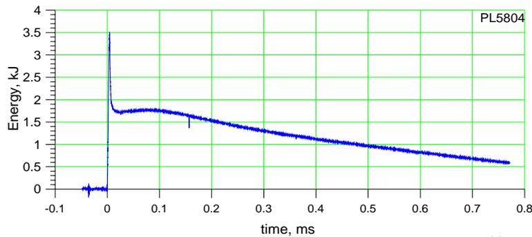
Fig.2. Energy stored in plasma with density of  $8 \cdot 10^{20} \text{ m}^{-3}$ .
