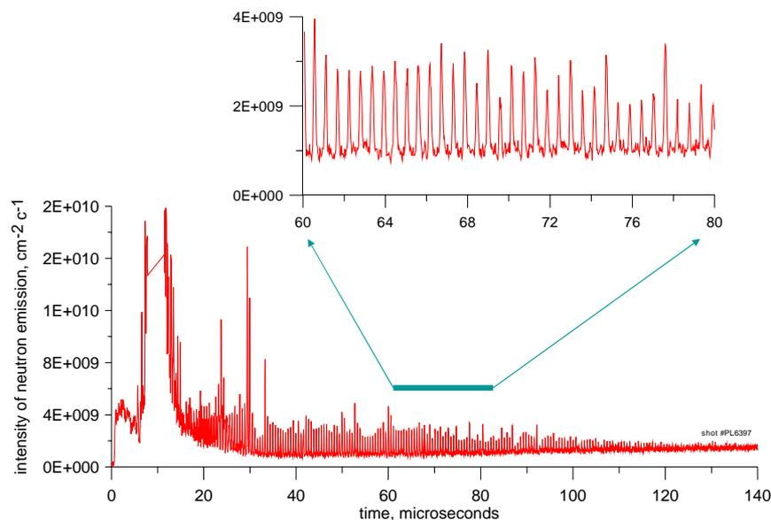
Fig.4. Initial phase of the neutron emission, there is almost no neutron flux during initial stage of the plasma heating. Then, approximately at the moment of emergence of the large density fluctuations, an intense neutron flash appears which is followed by a quasi steady neutron emission up to  $\sim 1$  ms. Periodical oscillations of neutron emission are shown.
