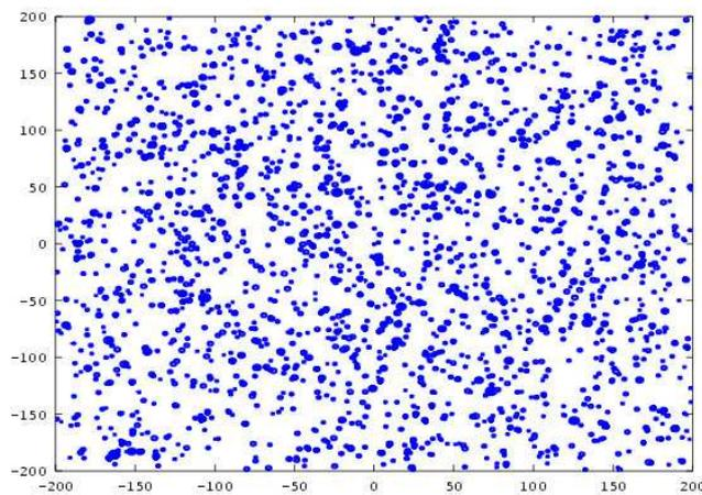
Fig.1 The steel surface after finish of fluctuation stage of blistering is shown. Colour indicates imperfections of surface: blisters covers and craters which were formed when bubbles destroyed on surface. Space coordinates  $x$  (abscissa axis) and  $y$  (ordinate axis) are measured in lattice parameters of steel.
