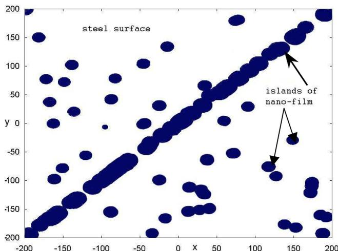
Fig.2 presents the surface of steel substrate with linear dislocation at time of fluctuation stage finish. The dislocation equation is  $y=x$ . Space coordinates  $x$  (abscissa axis) and  $y$  (ordinate axis) are measured in lattice parameters of steel.
