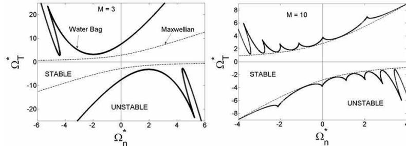
Figure 2: Dependence of  $\Omega_T^*$  on  $\Omega_n^*$  at the threshold for  $M = 3$  and  $M = 10$ . The dashed and solid lines correspond respectively to continuous and Water Bag distribution functions.
