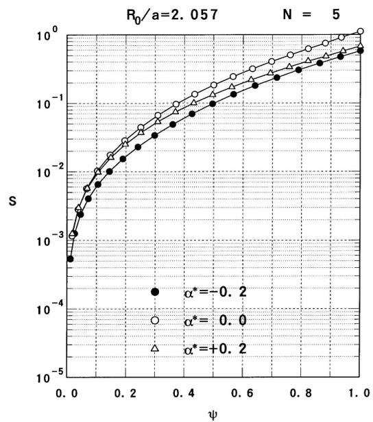
Fig.2 : Neo-classical Surface integrals for three type  $N=5$  system devices.
