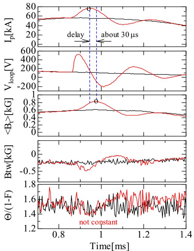
Fig.2: Time evolution of the RFP discharge with (red lines) and without (black lines) the oscillating of the toroidal electric field.
