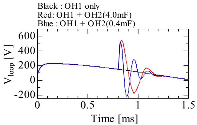
Fig.1: Time development of the toroidal loop voltage with and without the OH2 circuit.
