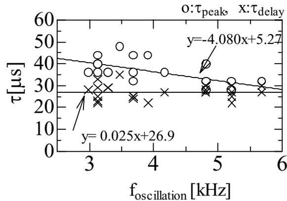
Fig.4: The dependence of the frequency of the oscillation of the toroidal plasma current on the delay times of the dynamo response.
