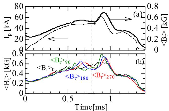
Fig.3: (a) Time evolution of the toroidal plasma current and averaged toroidal magnetic field. (b) The averaged toroidal magnetic fields at the different positions of the intervals of the 90-degree to the toroidal direction.
