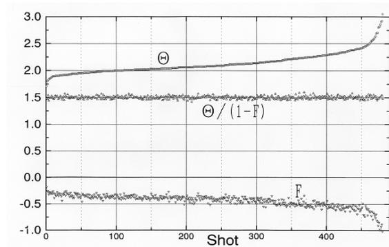
Fig. 1 The values of  $\Theta/(1-F)$  at the peak plasma current for normal RFP discharges having various  $\Theta$  values.
