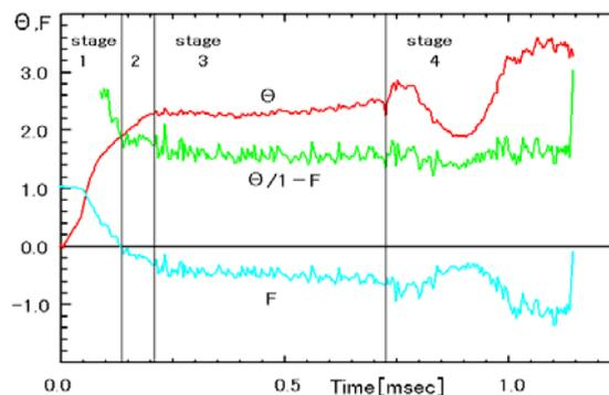
Fig. 2 The time history of  $\Theta$ ,  $F$  and  $\Theta/(1-F)$  values for a RFP discharge with additional oscillating E field.
