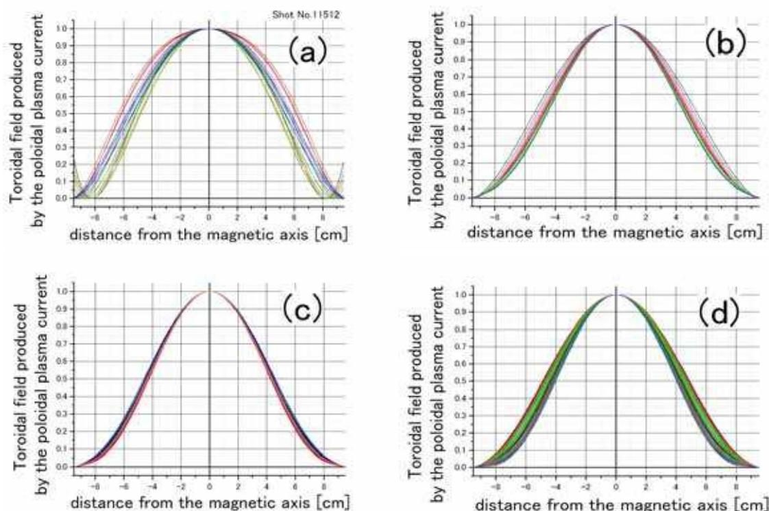
Fig.3. The time history of the radial distribution of the toroidal field produced by the poloidal current flowing in plasma in each stage; (a) before the RFP configuration, (b) RFP has constructed but  $F$  and  $\Theta$  are changing, (c)  $F$  and  $\Theta$  are constant but plasma current is increasing, (d) the large amplitude high frequency toroidal electric field is applied.
