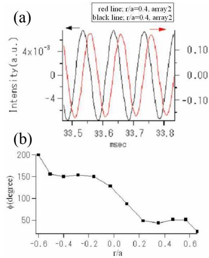
Fig.4: (a) The intensity of Fc with 10kHz at  $r/a = 0.4$  of array1 and array4. (b) The phase of the Fc with 10kHz.
