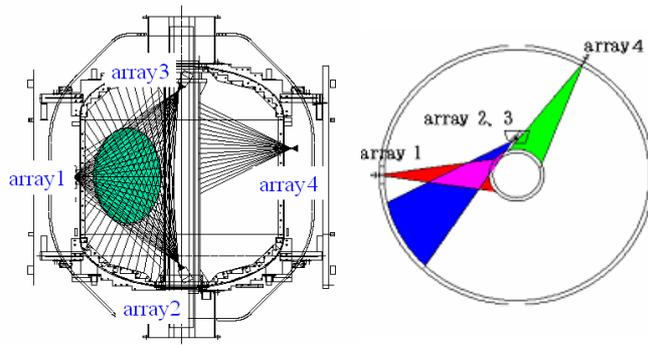
Fig.1: Left figure; poloidal cross diagram of the installation of each detector array and the line of sights of each detector. The ellipse represents a typical size of plasma. Right figure; toroidal cross diagram, measured regions of each detector array are painted.
