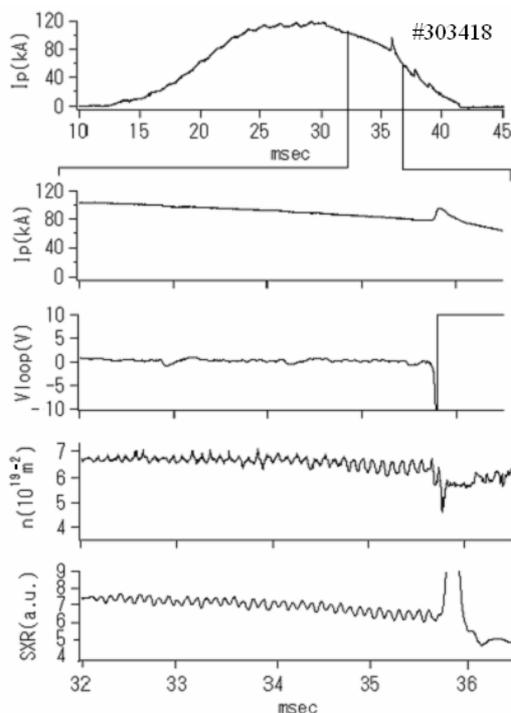
Precursor was observed during several milli-seconds before IREs. As shown in Fig.3(a), the frequency of SXR precursor was analyzed by fast Fourier transform (FFT) technique, and it turned out that the fluctuation had two dominant Fourier components ( $F_c$ ) with 10kHz and 4kHz.  $F_c$  with 10kHz and 4kHz were existed sometimes independently without IREs. The presence of both components with 10kHz and 4kHz leads to IREs.
