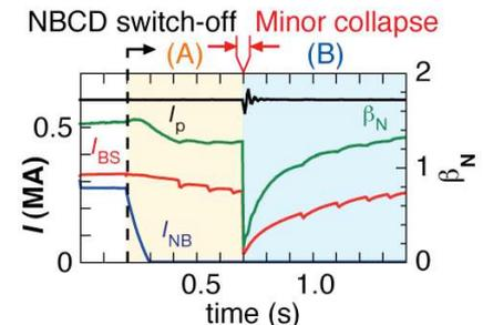
Fig. 3: TSC time-evolutions of normalized beta  $\beta_N$ , plasma current  $I_p$  and BS current  $I_{BS}$  after NBCD switch-off and following minor collapse phases (A), (B) in RS discharge (E42852).
