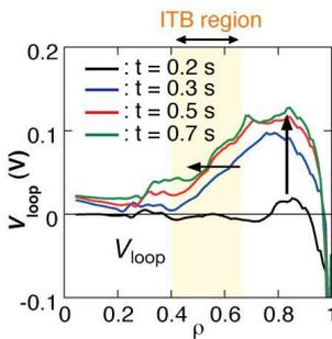
Fig. 5: TSC time-evolution of loop voltage  $V_{\text{loop}}$  profile in the first phase (A) ( $t = 0.2 - 0.7$  s). Induced loop voltage penetrates into ITB region on  $\tau_{\text{relax}}$  ( $\sim 600$  ms).
