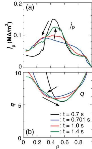
Fig. 7: TSC time-evolutions of (a) plasma current  $j_p$  and (b)  $q$  profiles in the second phase (B) ( $t = 0.7 - 1.4$  s). “Hyper resistivity” flattens plasma current and  $q$  profiles ( $t = 0.7005 - 0.701$  s). As BS current increases under continuous NB heating, plasma current profile becomes deeply hollow on  $\tau_E$ . And then,  $q_{\min}$  is decreasing and  $\rho_{q_{\min}}$  drifts towards the edge on  $\tau_E$ .
