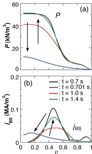
Fig. 6: TSC time-evolutions of (a) plasma pressure  $P$  and (b) BS current  $j_{\text{BS}}$  profiles in the second phase (B) ( $t = 0.7 - 1.4$  s). “Transport enhancement” leads to reduction of BS current as well as plasma pressure within 0.5 ms, as observed in JT-60U experiment. Under continuous NB heating, BS current increases in accordance with recovery of the plasma pressure on  $\tau_E$  ( $\sim 100$  ms).
