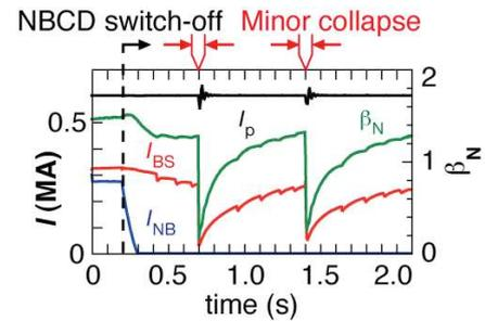
Fig. 8: TSC time-evolutions of normalized beta  $\beta_N$ , plasma current  $I_p$ , BS current  $I_{BS}$  and NB driven current  $I_{NBCD}$  after NBCD switch-off and following intermittent minor collapse of non-inductive RS plasma (E42852).  $\beta_N$  is almost recovered to that before collapse as observed in JT-60U experiment.
