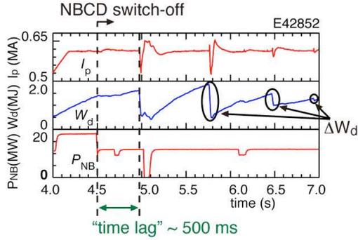
Fig.1: Waveforms of JT-60U non-inductive RS discharge (E42852): (a) plasma current  $I_p$ , (b) stored energy  $W_d$ , (c) total NB power  $P_{NB}$ . Notice that intermittent collapse occurred at 5.0, 5.8, 6.5 and 6.9 s after NBCD switch-off ( $t = 4.5$  s). There was time lag ( $\sim 500$  ms) between NBCD switch-off and onset of the first collapse.
