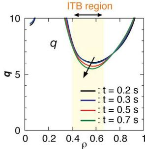
Fig. 4: TSC time-evolution of  $q$  profile in the first phase (A) ( $t = 0.2 - 0.7$  s). “Return” current penetration into ITB region leads to further lowering of  $q_{\min}$  together with inward drift of  $\rho_{q_{\min}}$  on  $\tau_{\text{relax}}$  ( $\sim 600$  ms).
