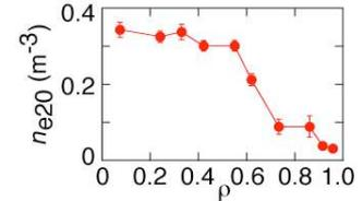
Fig.2: Plasma density profile at 4.85 s in Fig. 1. ITB exists at  $\rho \sim 0.6$ .
