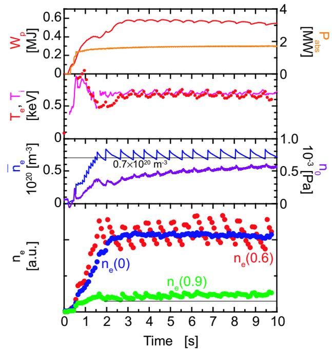
Figure 1: The temporal evolution of the key parameters in a repetitive pellet refueled discharge. The pellet firing interval is automatically controlled in real time to keep  $0.7 \times 10^{20} \text{ m}^{-3}$  at the pellet injection timing.
