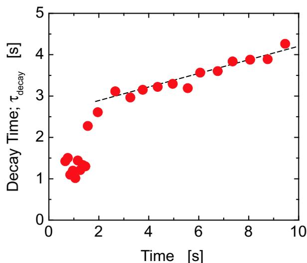
Figure 3: The change of density decay time in the density profile relaxation phase after pellet injection.
