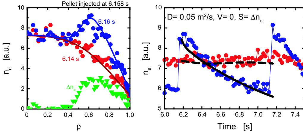
Figure 2: Comparison between measurement and simple diffusion calculation. The circles and lines denote the measurements and calculation results, respectively. (a) Measured and calculated density profiles change in the density profile relaxation phase after pellet injection. (b) Local electron density evolution at  $\rho = 0$  and  $\rho = 0.6$ .
