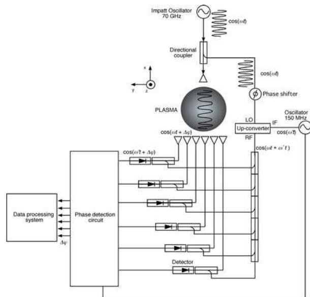
Figure 1. The schematic diagram of the multi-channel microwave interferometer system.
