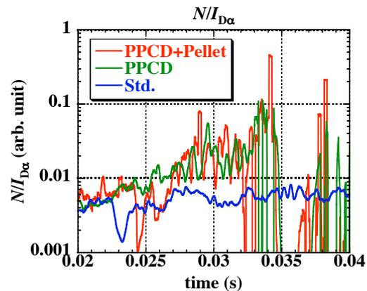
Fig. 4.  $N/I_{D\alpha}$ .  $N$  is total number of particles estimated from the density profile.  $I_{D\alpha}$  is total  $D\alpha$  emission measured by the toroidal monitor and the PSD.
