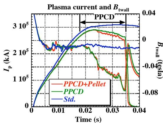
Fig.1 The plasma current and the toroidal magnetic field at the plasma edge. The PPCD started at  $t = 18 \text{ms}$ .
