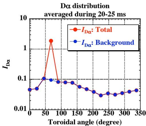
Fig. 3. Toroidal distribution of  $D\alpha$  emissions. The pellet injection port is at 67.5 degrees. The background emission at the 67.5 degrees is estimated using the background emissions at 45 and 90 degrees. The  $D\alpha$  emission at 67.5 degrees is measured by the PSD.
