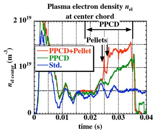
Fig. 2. Plasma density measured at center chord. The pellet is injected at  $t = 24 \text{ms}$ . The pellet is divided into two pellets during transferring.
