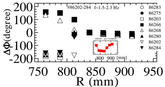
Fig.4 Phase difference along  $R$  for transport oscillations. Inset is the  $R$ -profile of the spectrum power at the perturbation frequency.
