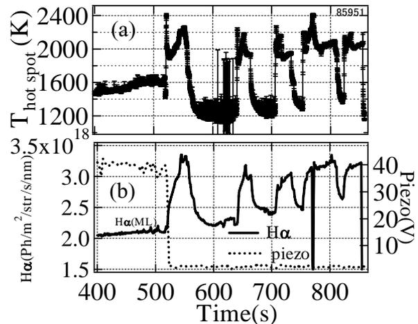
Fig.5 Localized heat load deposition on ML; (a)  $T_{hot}$ , (b)  $H\alpha$  from ML and the waveform of the gas puffing
