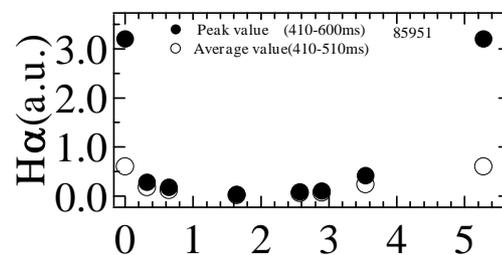
Fig.6 The global structure of the recycling around the torus. The zero position on the horizontal axis corresponds to the ML. The open and closed symbols before and during the first heat perturbation.
