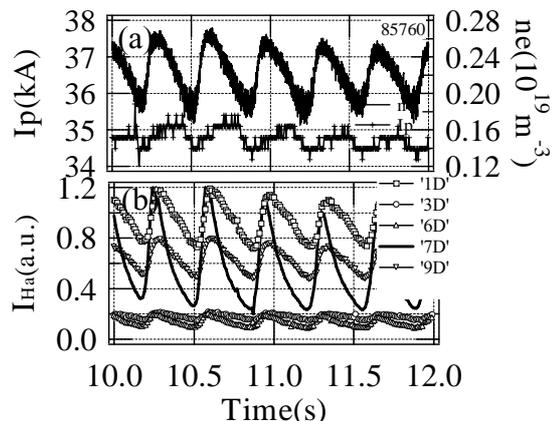
Fig.1 gas puff modulation: (a)  $I_p$  and  $n_e$ , (b)  $H_\alpha$  at various toroidal positions.
