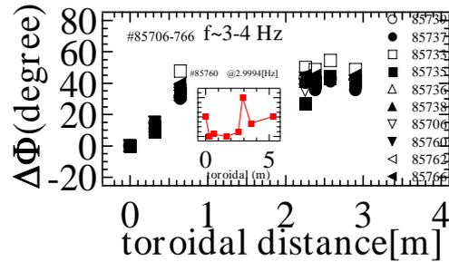
Fig.2 Phase difference along the toroidal direction. Inset is the toroidal profile of the spectrum power at the modulation frequency. The peak corresponds to the gas port.
