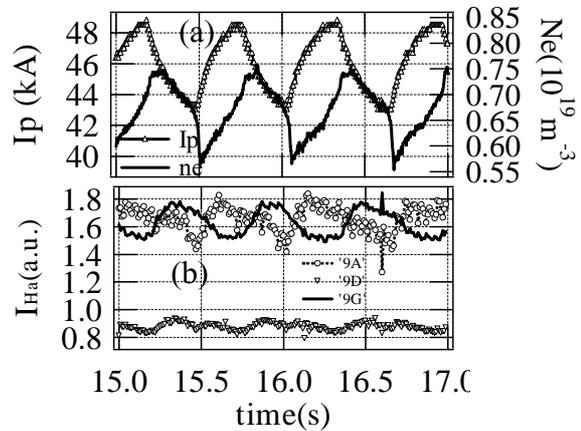
Fig. 3 Transport oscillations. (a)  $I_p$  and  $n_e$ , (b)  $H_{\alpha}$  at PL, inner (A: circles), center D: (triangles), and outer (G: solid line)
