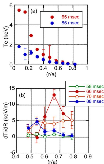
Fig. 5 (a) Electron temperature profile and (b) ion temperature gradient in ITB discharge.
