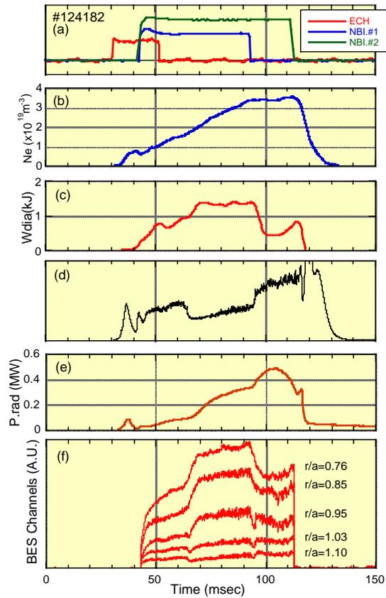
Fig. 1 Global parameters of H-mode discharge: (a) timings of heating, (b) line-averaged density, (c) diamagnetic energy, (d)  $H\alpha$  emission, (e) radiation power and (f) BES signals.
