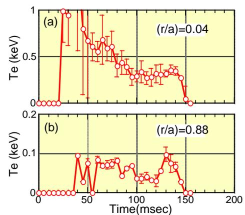
Fig. 4 Time variation of core and edge electron temperature.
