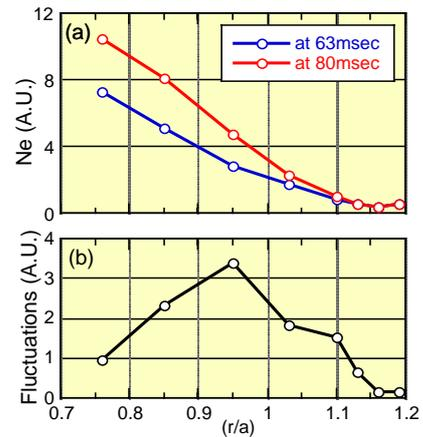
Fig. 2 Development of local density gradients and RMS profile of EHO oscillation.
