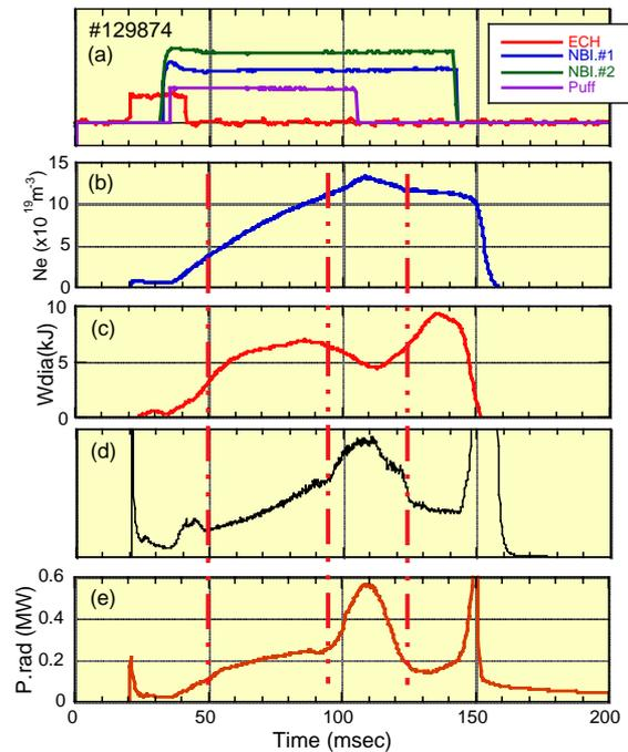
Fig. 3 H-mode discharge combined with reheat mode. Three dotted lines indicate H-mode transition, back transition and the second transition.
