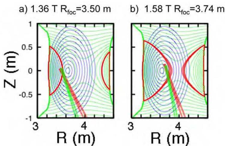
Figure 1: Vertically elongated cross section of Mod-B, flux surfaces, second harmonic resonance layers and ECRH beams for ripple a) top and b) bottom heating geometries.
