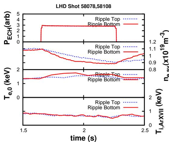
Figure 2: Temporal evolutions of line averaged density, central electron and ion temperature for ripple top (dotted lines) and the density at several spatial points b), and d) for bottom (thick lines) ECRH on NB heated ripple top [ a) and b) ] and bottom [ c) and d) ] discharge.
