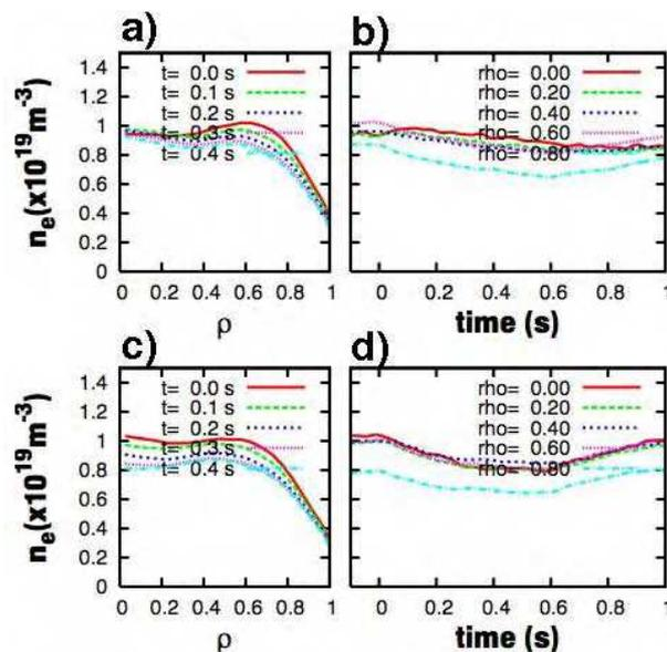
Figure 3: Density profile at several time slices after ECH injection [ a) and c) ]. Time evolutions of density at several spatial points b), and d) for heating cases.
