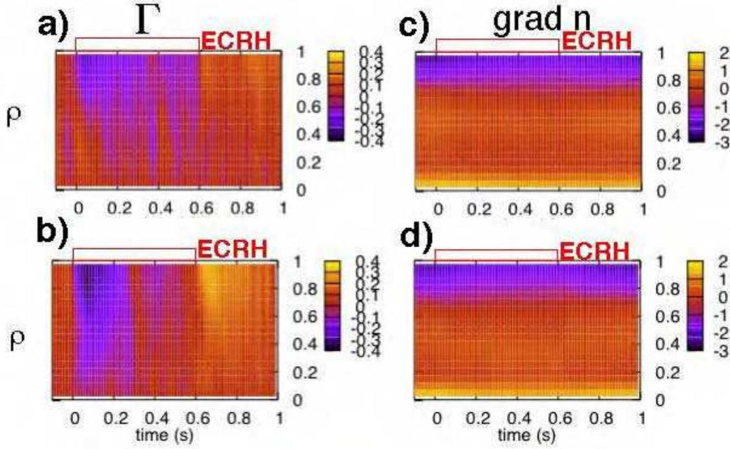
Figure 4: Particle flux deduced from Eq. (3) for ripple a) top and b) bottom cases. c) and d) show a temporal change in the density gradient for each case.
