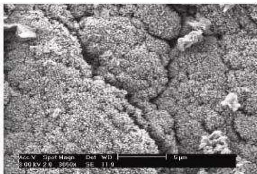
Fig.4 SEM micrograph of cauliflower-shape hydrocarbon film.
