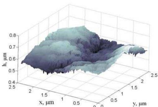
Fig.5. STM image of hydrocarbon film's surface deposited on the vacuum chamber.
