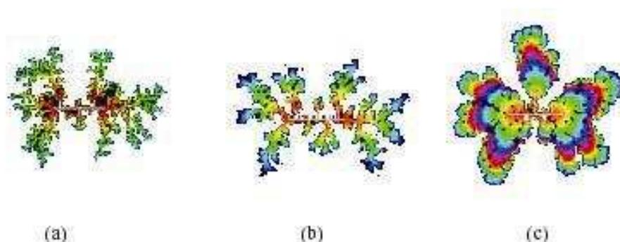
Fig.9 Diffusion limited aggregation with a variation in statistics of deposited particle diffusion. Simulation with Hurst exponent of diffusion: (a)  $H=0.5$ , (b)  $H=0.6$ , (c)  $H=0.8$ . Generations of the deposited particles are shown in different color.
