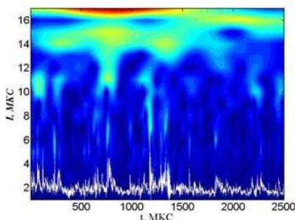
*Fig. 1.  $I_{\text{sat}}$  (white line) and its wavelet decomposition. SOL,  $r=34$  cm.*
