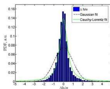
Fig.6. Probability density function (bars) of height's increments (normalized by standard deviation) shown in Fig. 5. Gaussian fit (dashed) and Cauchy fit (dashed-dot).
