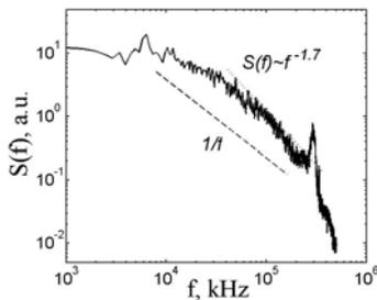
Fig. 2. Power spectrum of the particle flux fluctuations, SOL,  $r=34$  cm.
