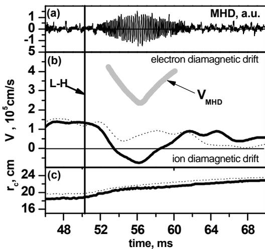
Fig. 2 Time evolutions of (a) magnetic probe signal, (b) MHD poloidal velocity (gray line) and Doppler velocities for discharges nearly without MHD activity (dotted line) and with strong MHD burst, (c) cut-off radius
