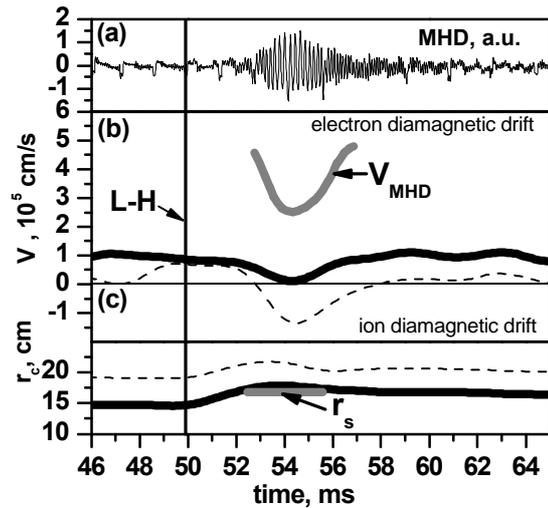
Fig. 3 Time evolutions of (a) magnetic probe signal, (b) MHD poloidal velocity (gray line) and Doppler velocities for microwave frequencies 19.45 GHz (dashed line) and 25.61 GHz (solid lines)
