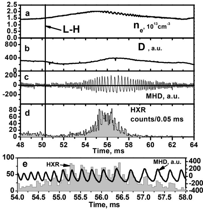
Fig. 4 Time evolutions of the signals (a) line averaged plasma density, (b)  $D_{\alpha}$  emission intensity, (c) magnetic probe signal, (d) and (e) HXR intensity with 0.05 ms integration time
