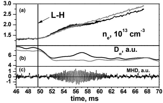
Fig. 1 Time evolutions of the signals measured in a shot virtually without MHD activity (gray lines) and in a shot with a sharp MHD; (a) line averaged plasma density measured along central chord, (b)  $D_\alpha$  emission intensity (c) magnetic probe signal
