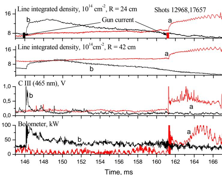
Fig.3: Waveforms of plasma discharge parameters in Globus-M under plasma jet injection; a- fresh grains loaded before each shot; b-fresh grains loaded before series of shots
