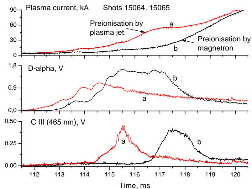
Fig.4: Time dependence of parameters in Globus-M at plasma discharge initiation; a-with plasma gun; b-with gas puffing and RF-preionisation.
