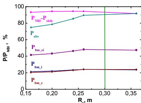
Fig. 3. NB absorbed power versus impact radius.  $P_{NB} = 0.6 MW$ ,  $I_p = 0.25 MA$ ,  $n_e = 3 \times 10^{19} m^{-3}$
