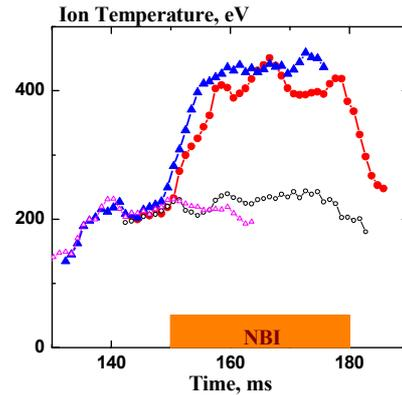
Fig. 4. Ion temperature evolution in shots #16776 (blue,  $R_s=30$ cm) and #17023 (red,  $R_s=33$ cm)  $P_{NB} = 0.35$  MW,  $E_{NB} = 23$  keV,  $I_p = 0.2$  MA,  $n_e = (2-3) \times 10^{19} m^{-3}$
