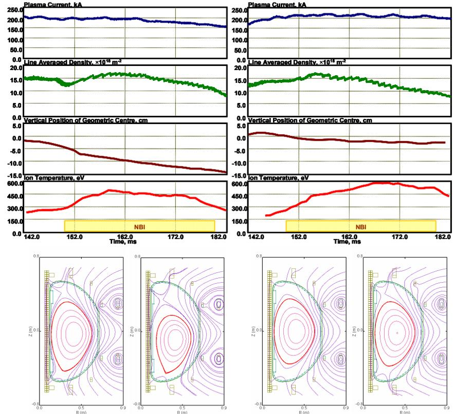
Fig. 2. Influence of plasma column shift on ion heating during NB injection in shots #11939 (left) and #17563 (right). Results of plasma magnetic surface reconstruction by EFIT code in the beginning and in the end of NB pulse are shown in the bottom.
