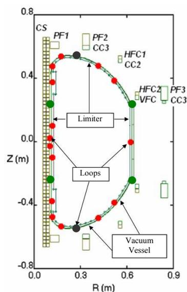
Fig. 1. Location of poloidal flux loops.
