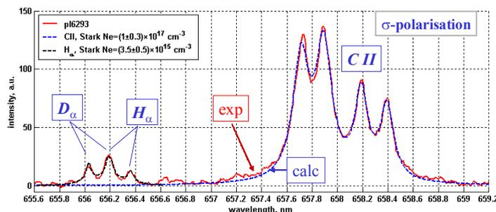
Fig.4. Example of a fit of observed spectrum.
