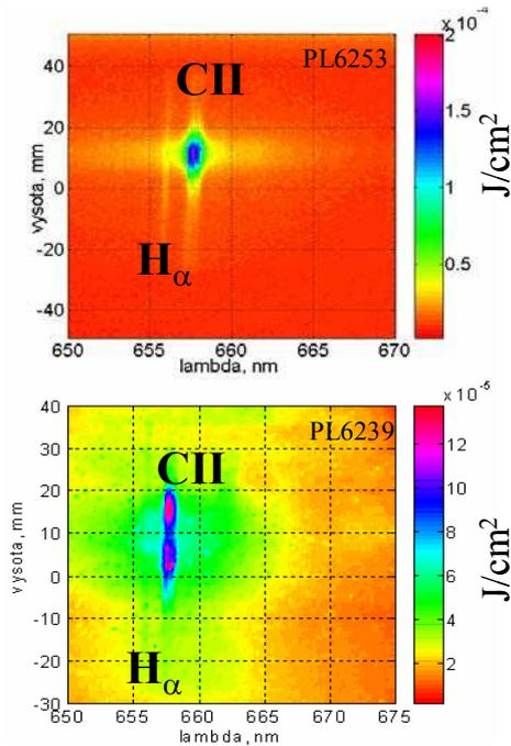
Fig.3. Spatially-resolved spectra: top – directly from the pellet surface, bottom – at some distance from the pellet. Pellets were positioned at +10 mm.
