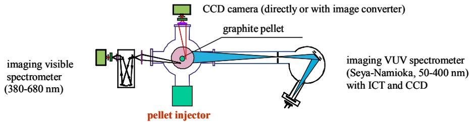
Fig.1. Layout of the pellet injection experiment (cross-section at pellet location).
