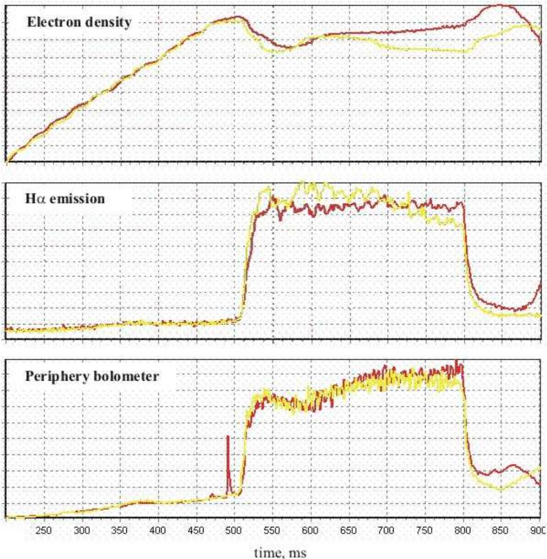
Fig. 1. Evolution of main plasma parameters in the reference shots before (#42312 red curve) and after (#42319 yellow curve) series with Li injection. All data are in arbitrary units.
