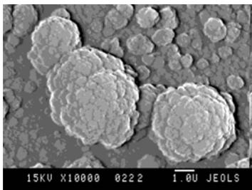
Fig.2 Dust particles after W macrobrush erosion
