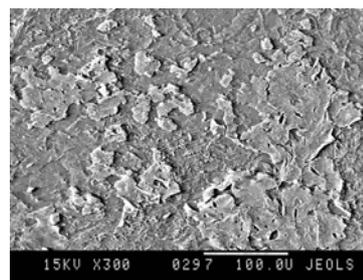
Fig.4 Flakes after CFC macrobrush erosion
