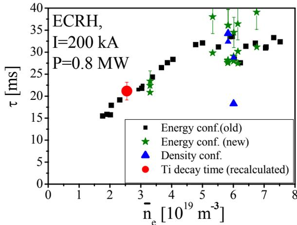
Fig.2 Confinement vs. density for ECRH 200 kA discharges.
