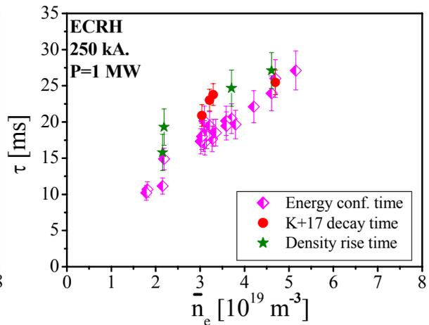
Fig.3 Confinement vs. density for ECRH 250 kA discharges.
