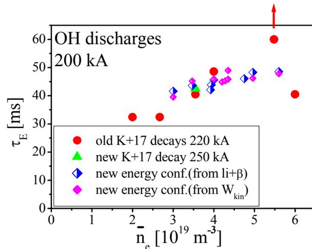
Fig.1 Confinement vs. density for OH discharges.
