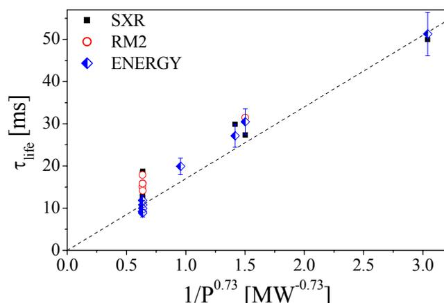
Fig.4 Ti impurity life time dependence from total ECRH power in discharge.
