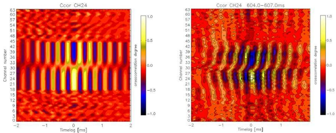
Fig.3: Comparison of cross-correlation contours for an artificial case of a rotating island (left) and  $k>1$  components of the SXR data (right). The channel 24 is reference.
