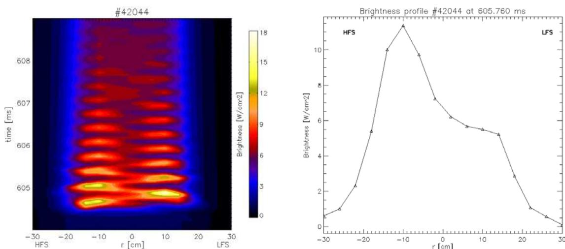
Fig.1: A snake-like structure visible on raw AXUV signals several milliseconds after the Ti pellet injection: contour plot (left) and the brightness profile at the selected time (right).
