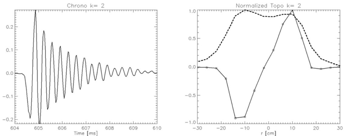
Fig.2: SVD of AXUV data. Chrono and topo of the  $k=2$  component corresponding to the island rotation. The dashed line represents the main plasma profile ( $k=1$ ).
