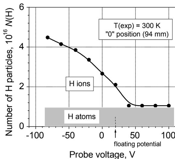
Fig. 3. Dependence of hydrogen accumulation on ion energy
