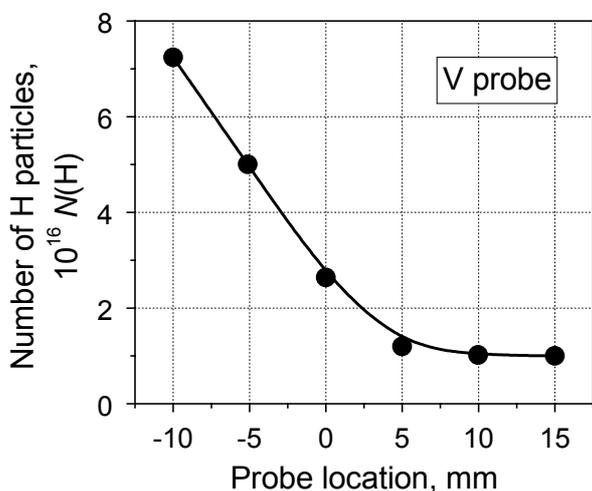
Fig. 1. Dependence of hydrogen accumulation on probe location.
