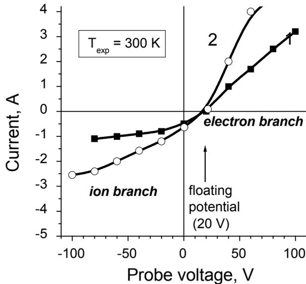
Fig. 2. Dependence of the ion current onto the absorption probe bias voltage for two radial positions of the probe (see also fig. 1).
