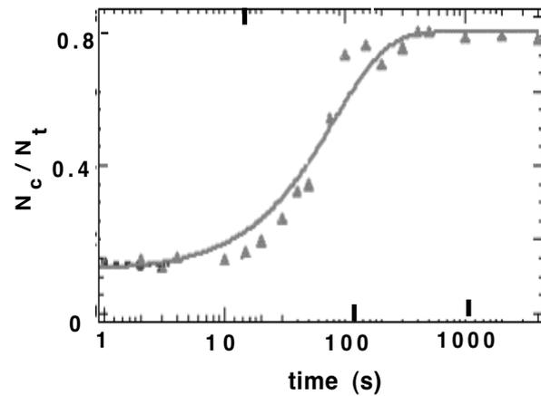
Fig.4 Increase of the ratio  $N_c / N_t$  during the compression. Here,  $f=9.15$  MHz,  $B_e = 0.34$  T and  $N_t = 6 \times 10^7$ .
