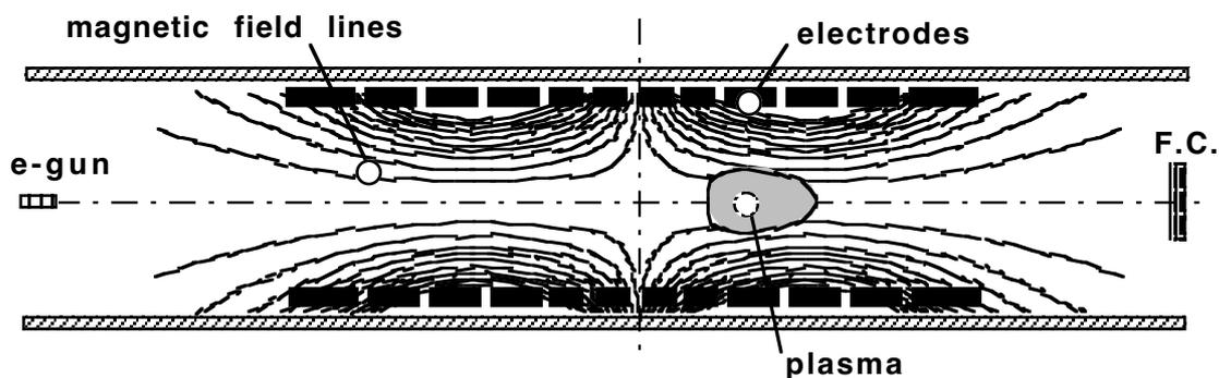
Fig. 2 Cross-sectional view of the setup inside the vacuum tube.
