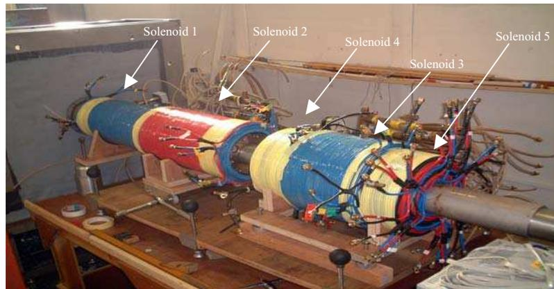
Figure 1: View of the solenoid configuration
