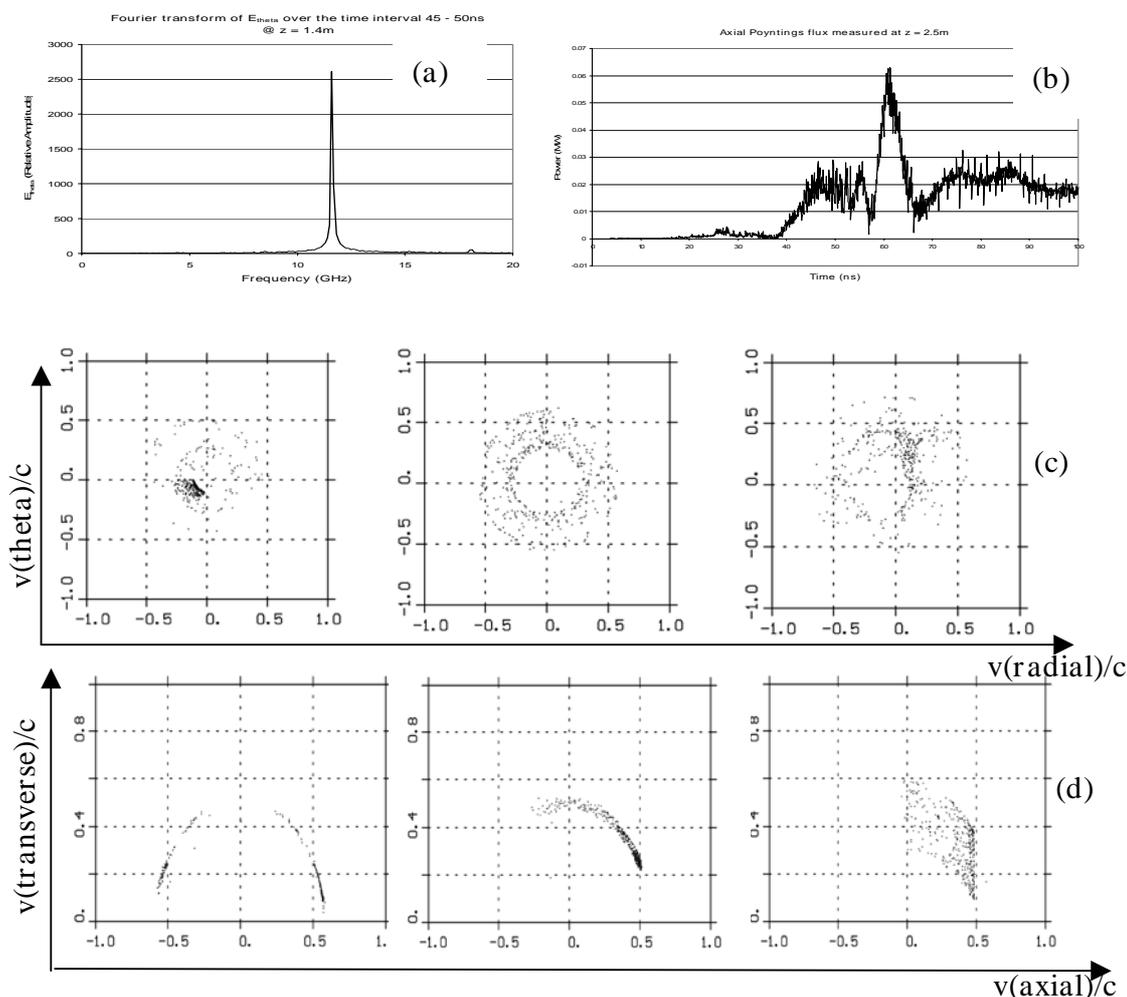
Figure 3: (a) Prediction of operating frequency, 11.7GHz, (b) Microwave output power (mirror ratio of 34), (c) Illustration of phase space bunching of electron orbits, (d) Evolution of the electron distribution function
