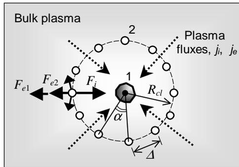
FIG. 3. Scheme of cluster: 1 – central big particle, 2 – small bound particles; dotted arrows – plasma fluxes.  $F_i$  – attractive ion drag force;  $F_{e1}$  and  $F_{e2}$  – electrostatic repulsion from the central and the neighbor particles, respectively.
