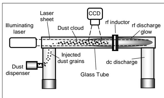
FIG. 1. Scheme of the PK-4 plasma chamber and experiment on cluster formation.
