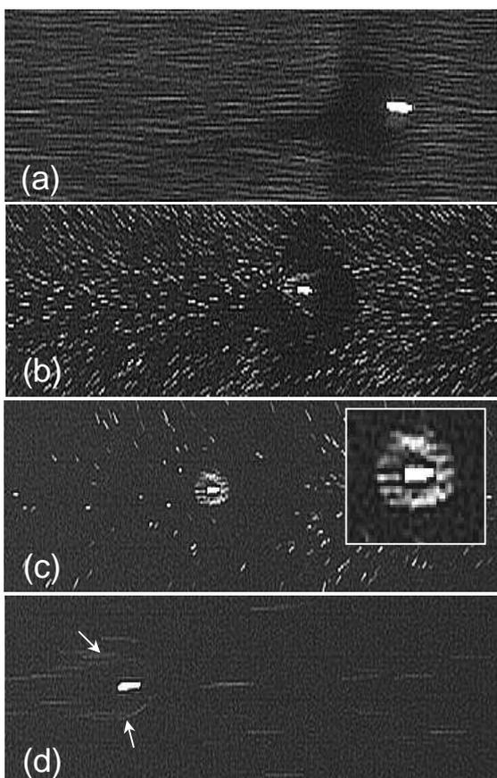
FIG. 2. Cluster formation and destruction in the central part of the discharge tube. (a) Dust cloud in uniform positive dc column before the rf pulse; (b) 60 ms after the rf pulse ignition: beginning of the cluster formation; (c) 120 ms after the rf pulse ignition: formation of cluster is complete; (d) 180 ms after the rf pulse ignition: rf pulse is finished, cluster is disrupted instantaneously. Area shown is about  $7 \times 3 \text{ mm}^2$ .
