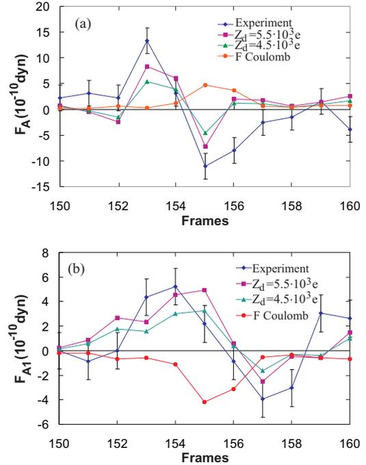
Figure 1: Vertical projections of the force acting on the cluster particles A and A1 during the distortion phase.
