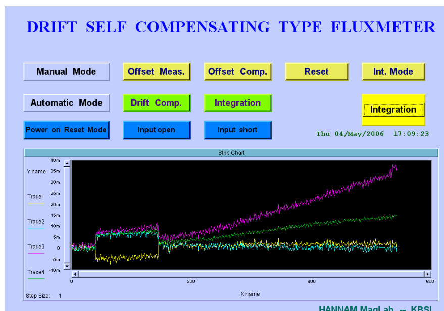
Fig. 1. Digital signal monitored by a program in a PC controlling the integrator.
