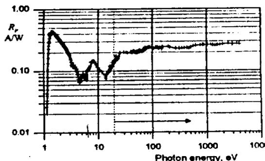
Fig 1: AXUV PD spectral response.
