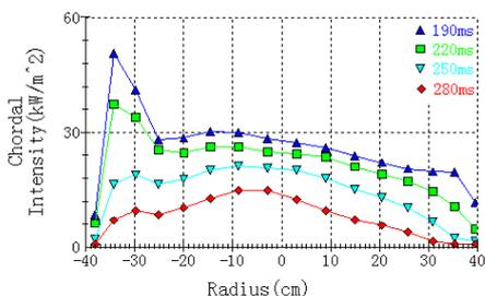
Fig3: the radiation profiles on the single null divertor operation on HL-2A. (shot 1654 , flat top:  $I_p=139kA$  ,  $n_e=0.9 \cdot 10^{19} m^{-3}$ ).
