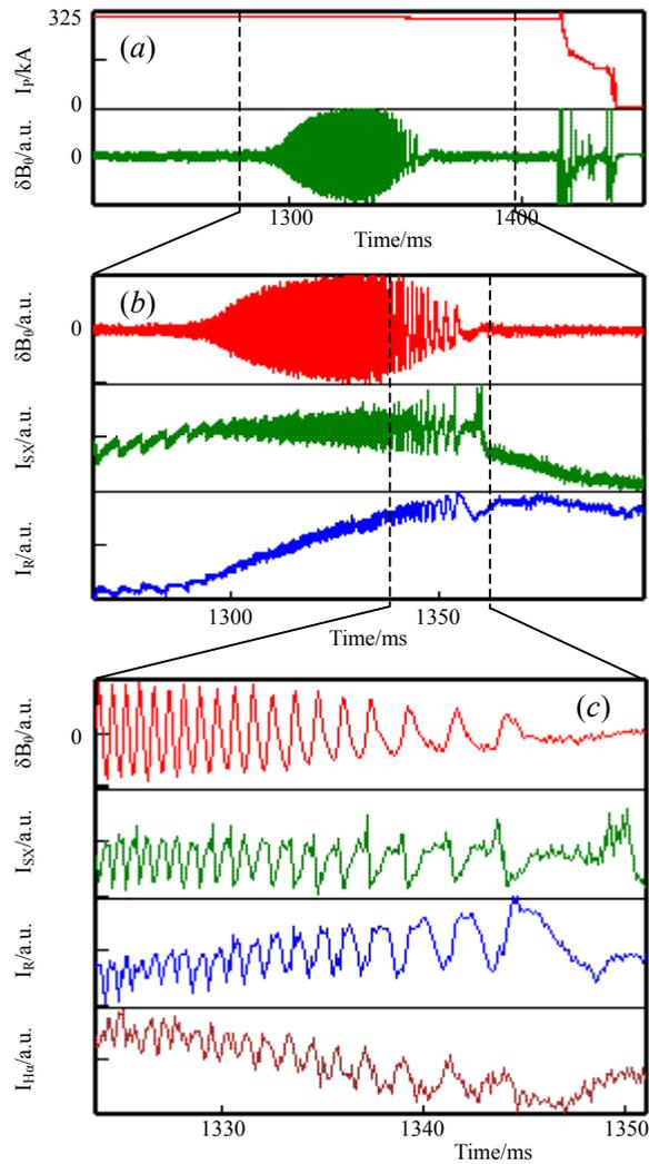
Fig5. Typical discharges before disruption. a)  $I_p$  and minrov signal  $\delta B_\theta$  before disruption. b) responding  $I_{SX}$  from Soft X ray,  $I_{rad}$  from the bolometer and  $I_{ha}$  from Ha measurement before disruption.
