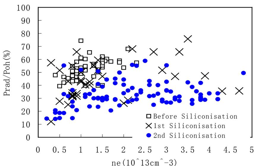
Fig4: the statistic results of the  $P_{\text{rad}}/P_{\text{ohmic}}$  over the line averaged density  $n_e$  on the limiter configuration.
