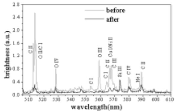
Figure 3 demonstrates variety of the signal strength of the ionization levels of impurities before and after wall siliconization
