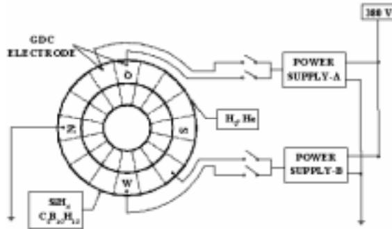
Fig.1. Glow discharge cleaning (GDC) system in HL-2A
