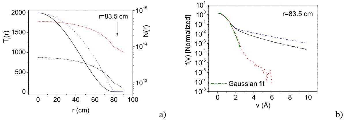
Figure 1: a) Density profiles (dashed-dotted black and short dash red, log. scale) and temperature profiles (solid black and dotted blue) used in the simulations. b) Calculated VDF at  $r = 83.5$  cm. The velocity is expressed in terms of the equivalent Doppler shift ( $\text{\AA}$ ) for the  $D\alpha$  line. The green dashed-dotted line is a Gaussian fit, giving a temperature very close to the local  $T_i$ .
