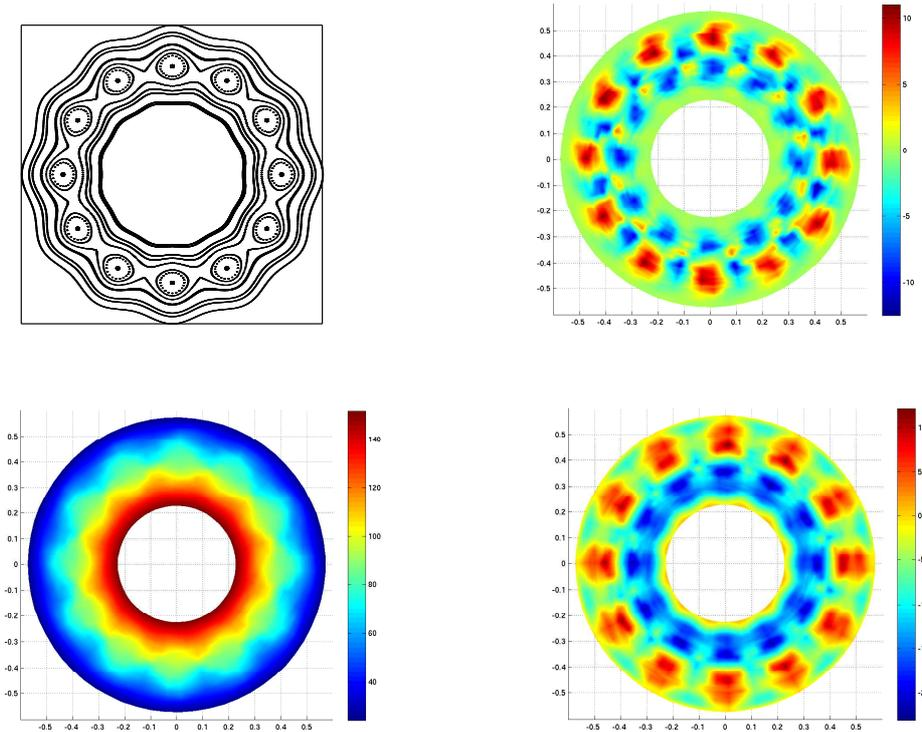
Figure 1: Poincaré-plot of the magnetic perturbation field (top left), poloidal profiles of the static density perturbation  $\bar{n}$  (top right), the background density + static perturbation  $n_b + \bar{n}$  (bottom left) and the difference  $\bar{n} - \bar{\phi}$  of the static density and electric potential perturbations.
