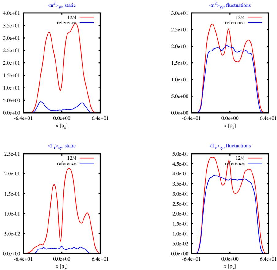
Figure 3: Radial profiles of the  $\theta$ - $\phi$ -averaged static density perturbations (top left), density fluctuations (top right), static radial  $E \times B$ -transport (bottom left) and radial  $E \times B$ -transport due to fluctuations. The red curves show the profiles of the perturbed plasma, the blue curves show the unperturbed case.
