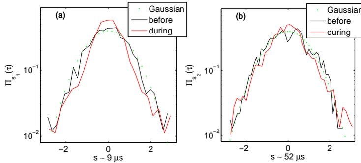
**Figure 2:** Semi-log plot of the PDFs of the signal measured in the SOL ( $r/a = 1.1$ ) for two different scales, normalized at mean 0, and variance 1. (a)  $s_1 = 9 \mu s$  and (b)  $s_2 = 52 \mu s$  before (in black) and during (in red) the DED. The dotted points indicate the best Gaussian fit.
