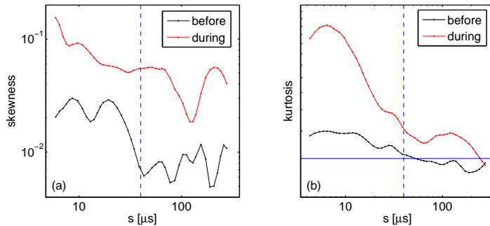
**Figure 3:** Log-log plot of (a) skewness and (b) kurtosis as a function of the scale. The  $S$  and  $K$  values in the plots are averaged over all radii in the SOL. The dashed lines mark the time scales around  $40\mu s$ .
