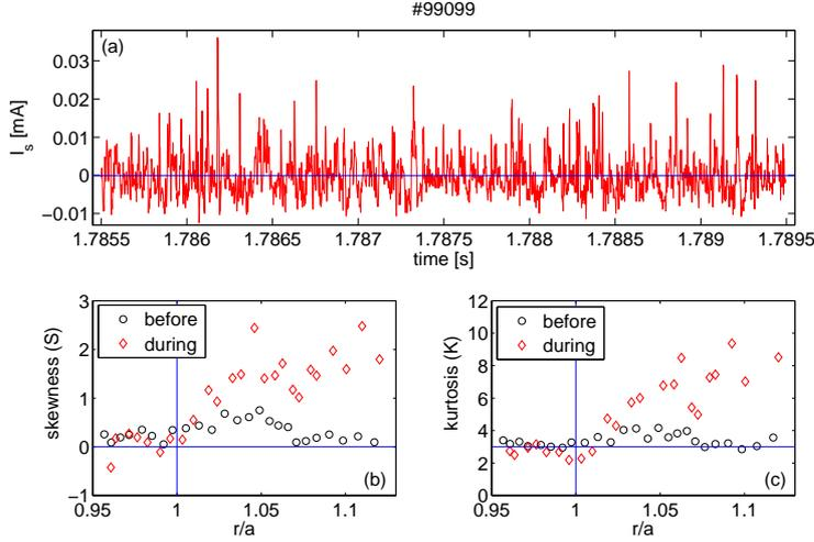
**Figure 1:** (a) Time trace of  $I_{sat}$  detected by a Langmuir probe during the DED phase at  $r \approx 50$  cm. Shown in (b) and (c) are the radial profiles of skewness and kurtosis of  $I_{sat}$  measured before (in black) and during (in red) the DED.
