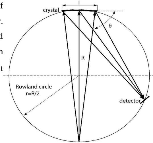
Fig. 1: Schematic of the spectrograph made in asymmetric Rowland geometry.
