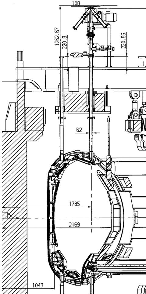
Fig. 2: Scheme of the spectrometer mount on AUG. total weight of about 10 kg. The spectrometer is mounted on the middle upper port in sector 2 of AUG (see Fig. 2) with the line of sight approximately going through the center of the poloidal cross-section.
