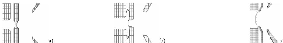
Fig. 5. Emission boundaries for different electrode configurations: a) cylindrical hole ( $\varnothing=1.5\text{mm}$ ), b) cylindrical with smaller diameter ( $\varnothing=1\text{mm}$ ), c) conic hole.
