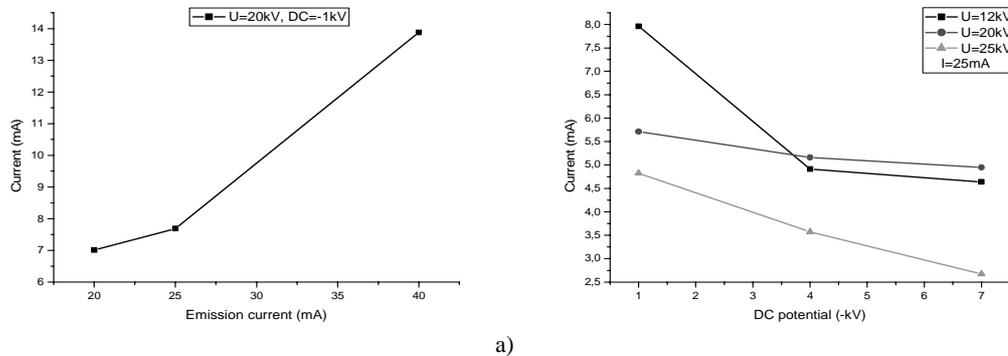
Fig. 3. Intensity of the ion beam at the end of section as function of the: a) emission current, b) dc-
